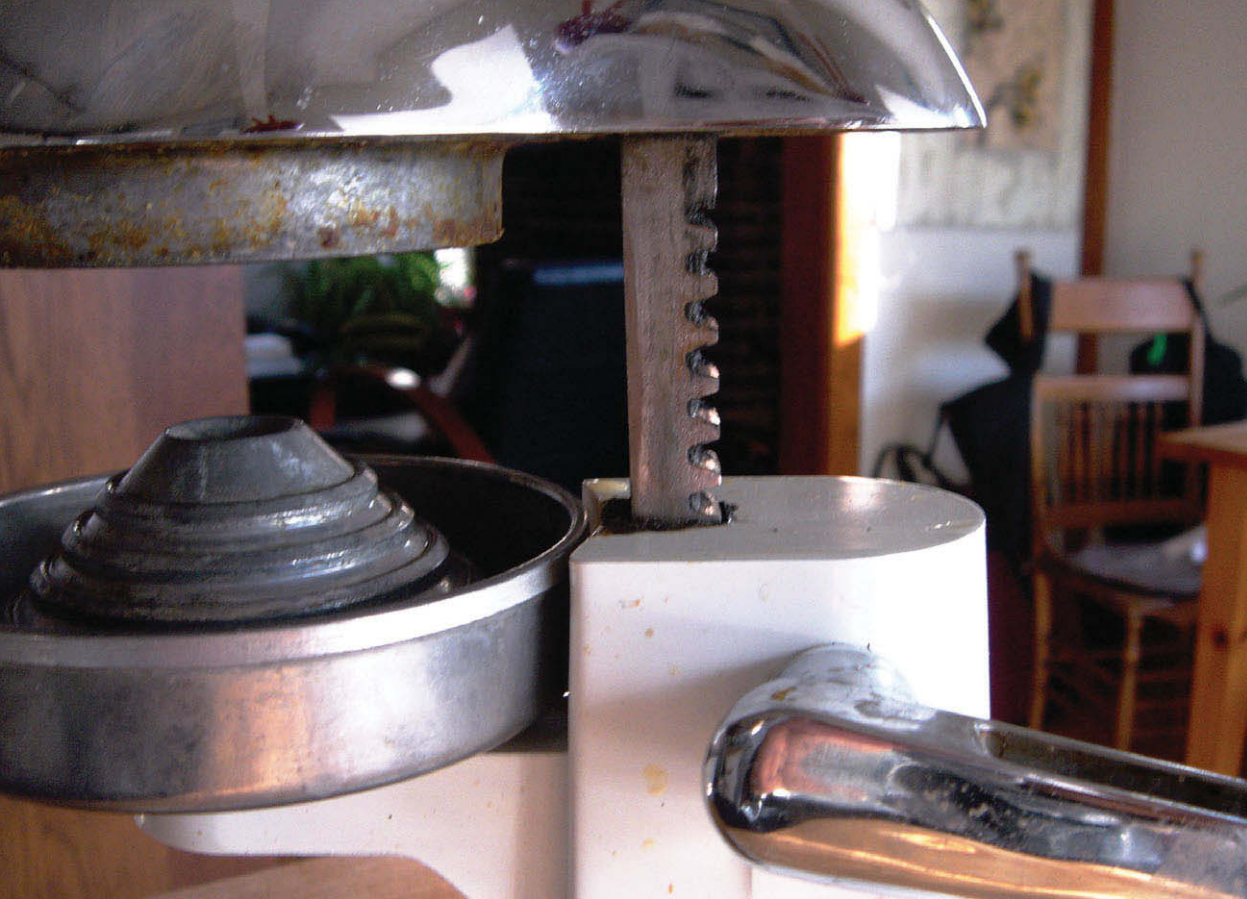
Figure 48: Gear Mechanism of the Mighty OJ
