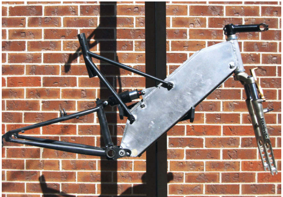
Figure 28: Engineering Prototype of Trek's Y-Bike
