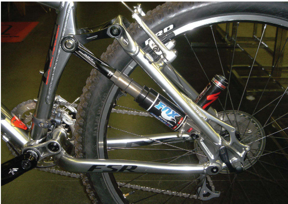
Figure 30: Specialized Epic Bicycle with Inertia Valve Shock
