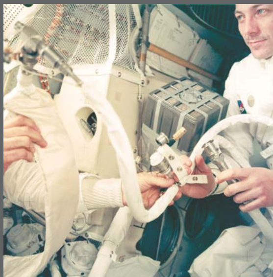
Astronaut John L. Swigert Jr., hooking up the adapted carbon dioxide filters.
